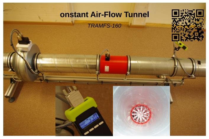
This is air-flow reference measure device. It keeps steady airflow through the tunnel and updates the flow-rate 2 times in second. Value is shown on graphical LCD display with back-light. With this device you can:
